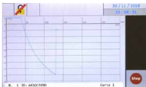
Real-time graph of the cryoscopic point measurement
