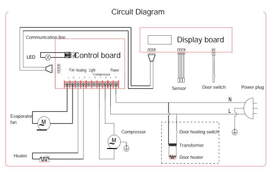
Note: The inside of the dotted frame is divided into optional parts, which are only applicable to products with door heating.
