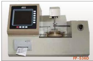
The instrument is designed and made as per the National Standard of People' Republic of China GB/T3536-2008 "Test Methods for Flash and Fire Point of Petroleum Products (Cleveland Open Cup Methods)". it is suitable to determine flash point and fire point of petroleum products having a flash point higher than 79 t, excepting fuel oils.
