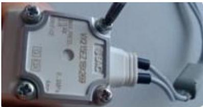
Remove the 4 screws of the solenoid valve.
