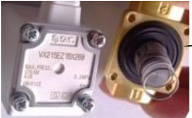
Lift the valve head vertically. Keep the spring stays on it.
