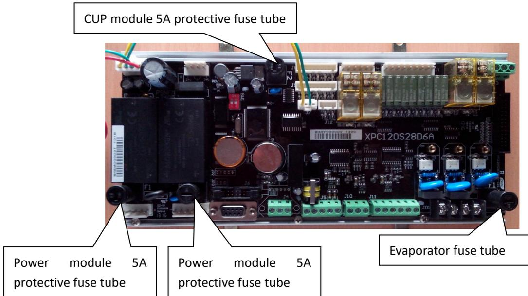
There are corresponding fuse in the equipment accessories , if there is a fuse burn out, find corresponding specification of fuse to replace it.
