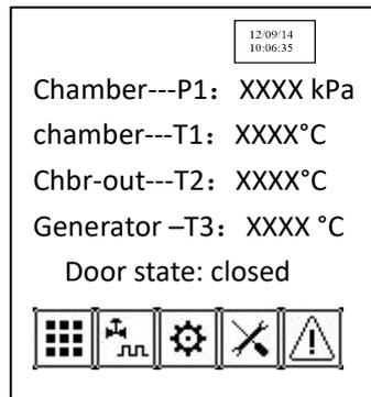
Chamber-P1: Indicates the chamber pressure
