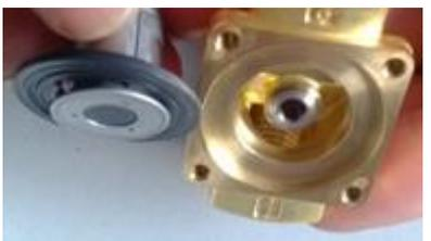
Take out the movable core and seal ring to view the sealing surface of the valve.
