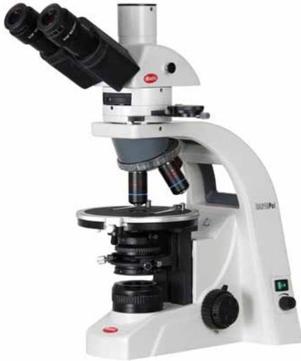
Motic **BA310Pol** microscope offers superb optical performance and flexibility in system expansion that can be applied to thin section petrography, mineralogy, industrial and medical applications.
